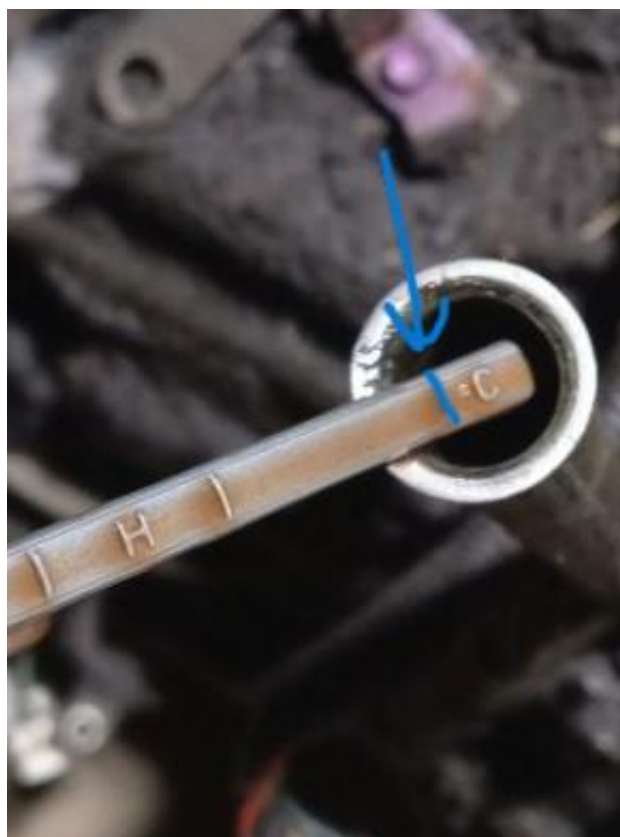
Figure.1 - Low oil level
