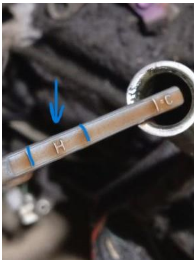
Figure.2 - Optimal transmission fluid level
