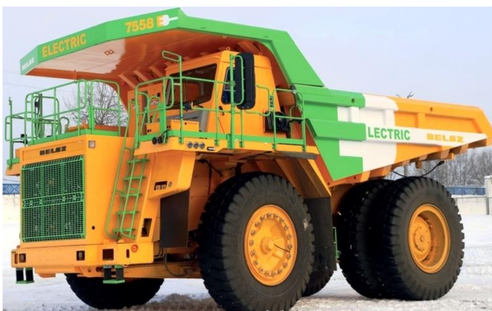
Fig. 1. Off-highway dump truck BelAZ-7558E of 90 t capacity
