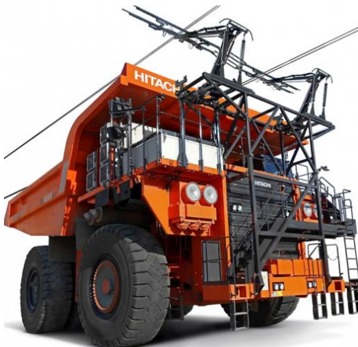
Fig. 2. Off-highway dump truck-trolleybus Hitachi EH4000 AC-3 of 221 t capacity [8]
