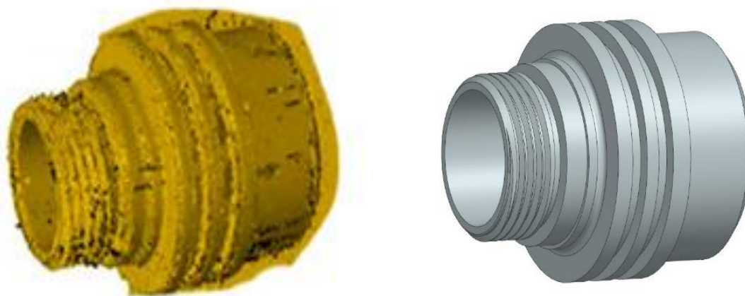
Fig 2. Reconstructing sample via point cloud.
